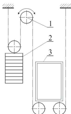
Fig. 3. Roping system of the analyzed lift
