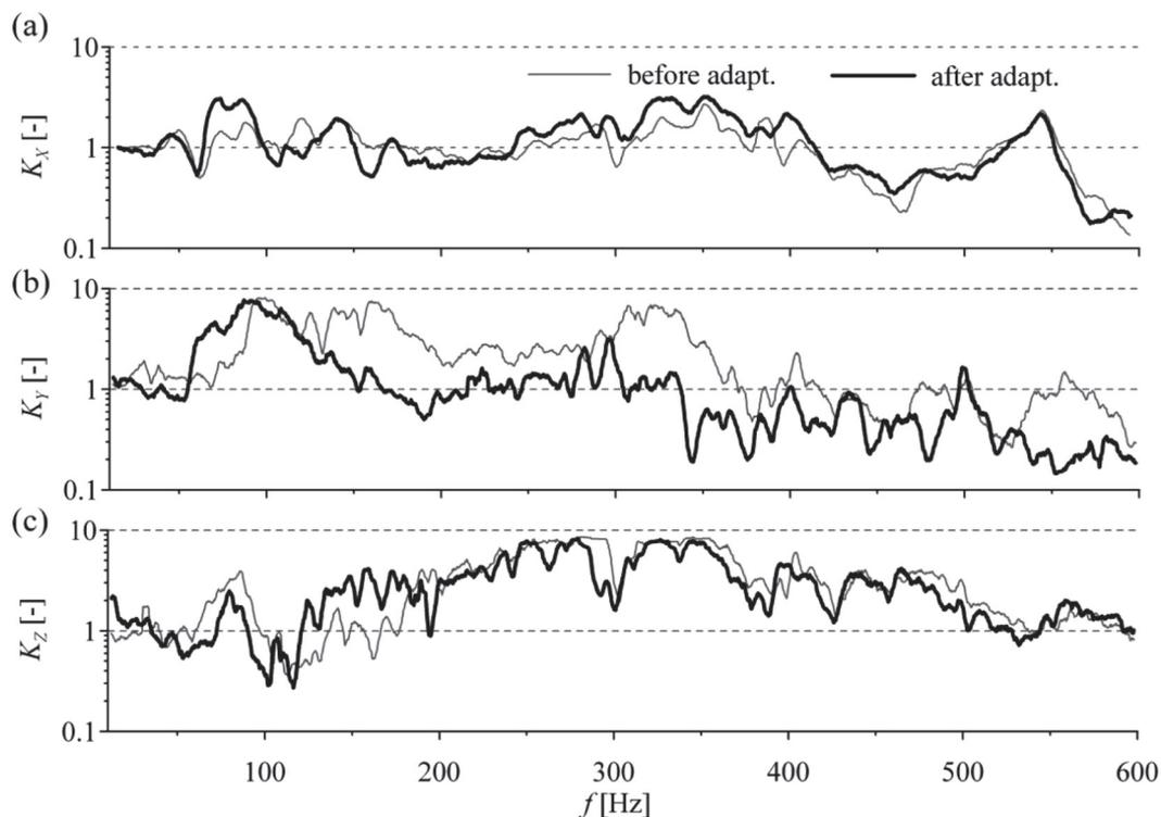
Fig. 10. The damping coefficient  $K$  in the function of frequency in the case of modified vibration isolation of the drive
