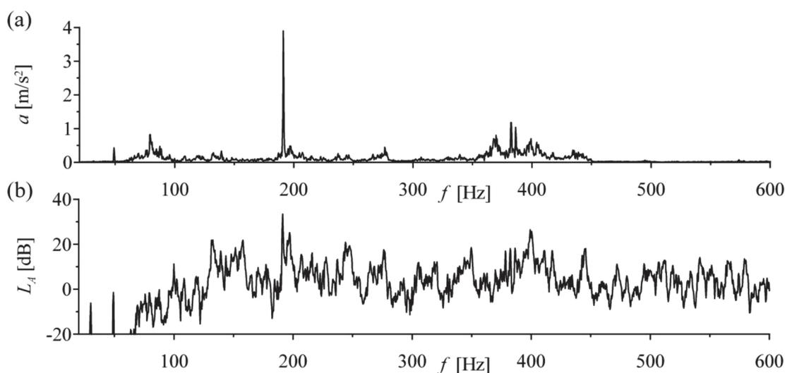
Fig. 8. Frequency components of sounds and vibrations in Room No 1- prior to the V-A adaptation (a) – acceleration values, (b) – sound level values
