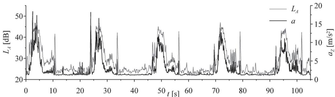
Fig. 9. Full duty cycle of the passenger lift- downward travel, registered in Room No 1
