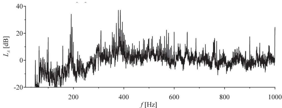
Fig. 7. Sound levels due to the hoist unit operation prior to the V-A adaptation- identification of frequency components
