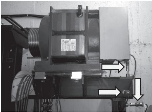
Fig. 5. Sensor positions on the steel support
