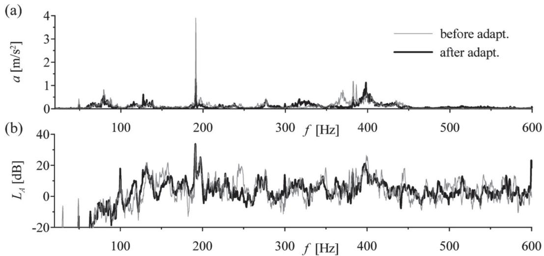
Fig. 12. Frequency analysis of sounds and vibration in Room No 1 after V-A adaptation
