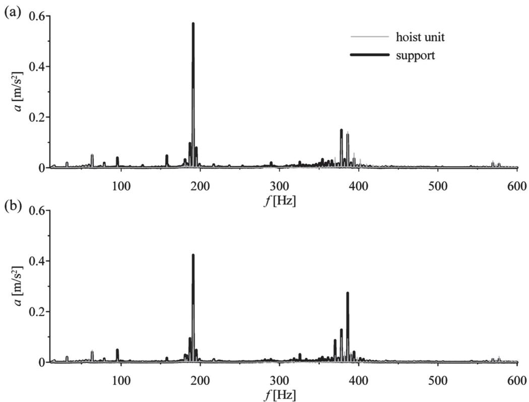
Fig. 6. Vibrations of the hoist unit prior to V-A adaptation
