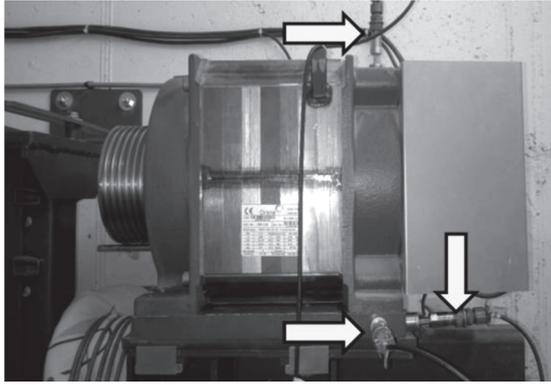
Fig. 4. Sensor positions on the drive unit
